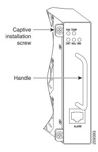
Step 2 Grasp the fan tray handle with one hand and the outside of the chassis with the other hand. Figure 3-12 shows the front of the fan tray, including the handle.
